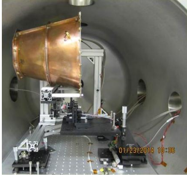
Figure 7. Tapered Cavity Test Article Mounted on Torsion Pendulum
